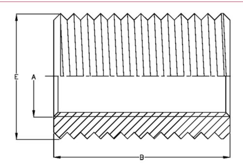
Female thread A = M12Length B= 18Male thread E= M16Type= 97x 000 120.120
